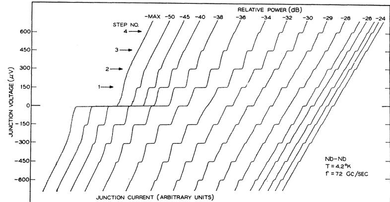
FIG. 1. Voltage-current curves for a Nb-Nb point-contact Josephson junction exposed to a 72-Gc/sec signal at various power levels.
