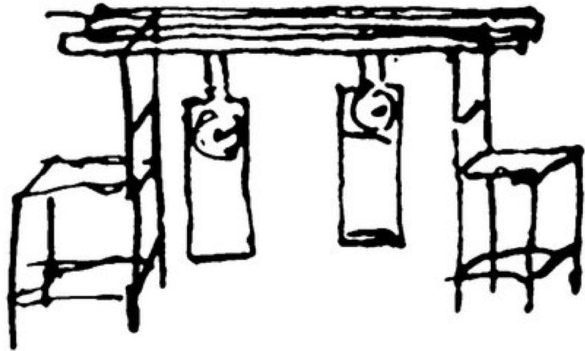
*... we suspended two clocks so constructed from two hooks imbedded in the same wooden beam ... the motions of each pendulum in opposite swings were so much in agreement that they never receded the least bit from each other ... the cause of this is due to the motion of the beam, even though this is hardly perceptible.*
